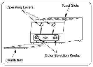
Figure 4. Controls and Crumb Tray
