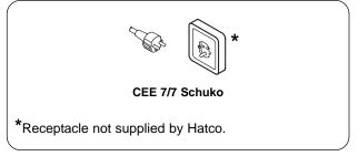
Figure 2. Plug Configurations
