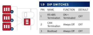
The DIP switches are used to provide a build-in termination to both the MJ2 port and CAN port if needed. The termination for these ports should only be used if this device is located at either end of the multidrop/daisy-chained RS-485 network or CAN bus.
