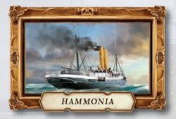
1881: The 4.247 GRT large HAMMONIA was already the third ship from HAPAG carrying this name, and was built in Glasgow. She was completely made of steel and divided into nine watertight sections. Be-cause of her unusual width, she had a high stability. Several steam-driven pumps propelled a fan system that supplied fresh air to all
